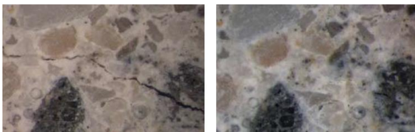
Figure 4 Concrete with Healing Agent before and after healing. The inside of the crack is clearly filled.
